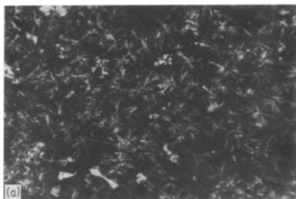
Figure 2 Optical micrographs of melt-crystallized films of iPP-1: T_c = (a) 129, (b) 135, (c) 139 ^{\circ}\text{C} .
