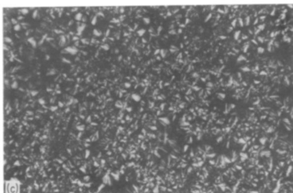
Figure 4 Optical micrographs of melt-crystallized films of GRiPP-3: T_c = (a) 129, (b) 135, (c) 139°C.
